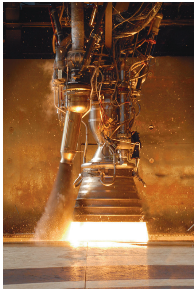
Nine SpaceX-built Merlin 1C engines power the first stage of Falcon 9. Each generates 115,000 lbs of thrust at sea level, providing over 1-million pounds of thrust to the vehicle upon liftoff.
